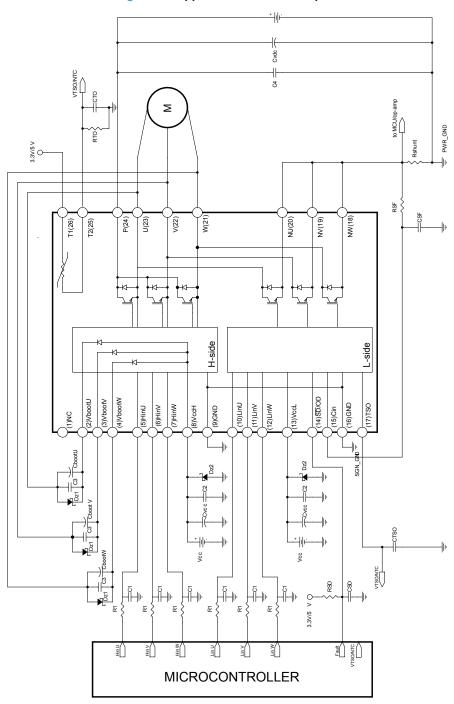
Figure 10. Application circuit example
