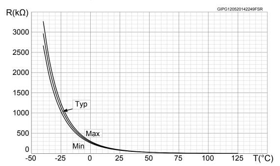
Figure 8. NTC resistance vs temperature
