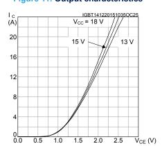
Figure 12. V<sub>CE(sat)</sub> vs collector current
