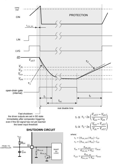
$R_{ON\_OD}$  =  $V_{OD}/5$  mA, see Table 10. Sense comparator ( $V_{CC}$  = 15 V, unless otherwise is specified);  $R_{PD\ SD}$  (typ.) = 5 V/I<sub>SDh</sub>
